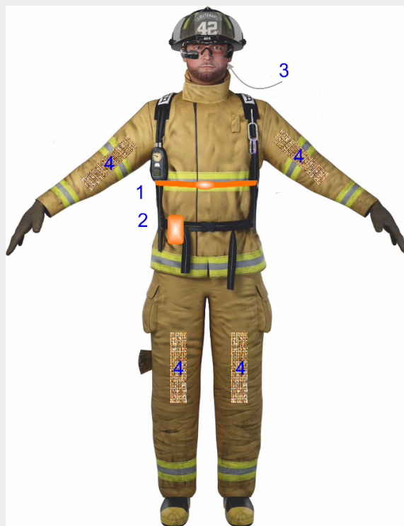
Figure 4: Firefighter Smart Clothing with life sensors (under clothing) - 1, center module - 2, augmented reality glasses - 3 and ferroelectric based energy harvester panels - 4.
